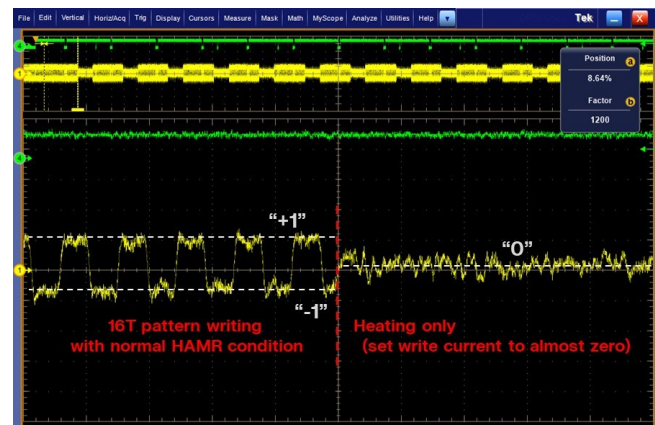
Fig. 1. Waveform (screen capture of digital oscilloscope) Bottom lefthand side: 16T pattern writing with normal HAMR condition. Bottom righthand side: Heating only.
