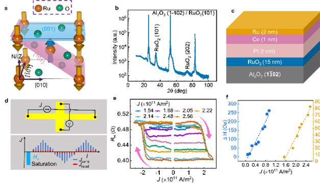
Fig. 1 (a) Crystal structure of  $\text{RuO}_2$  unit cell. (b) Gonio scan ( $\theta$ - $2\theta$ ) showing crystallinity of sputtered  $\text{RuO}_2$  film. (c) Schematic of stack structure. (d) Experimental schematic for SOT-driven switching. (e)  $R_H$  vs  $J$  switching loops at various ranges of  $J$ . (f) Variation of  $\Delta H$  and  $\text{SW}\%$  as a function of different applied  $J$ .
