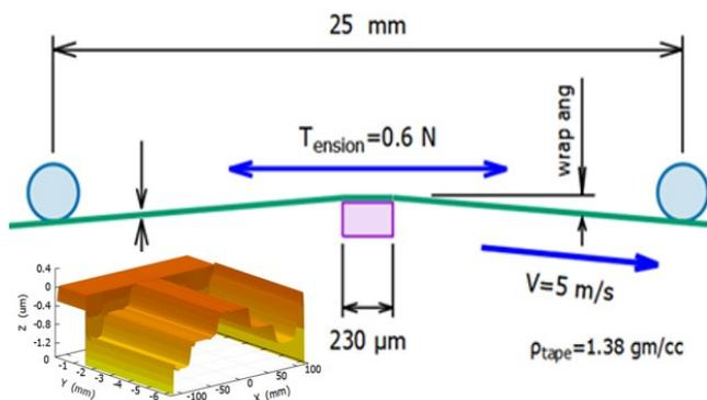
Fig. 1. Overall tape configuration and patterned tape bearing surface
