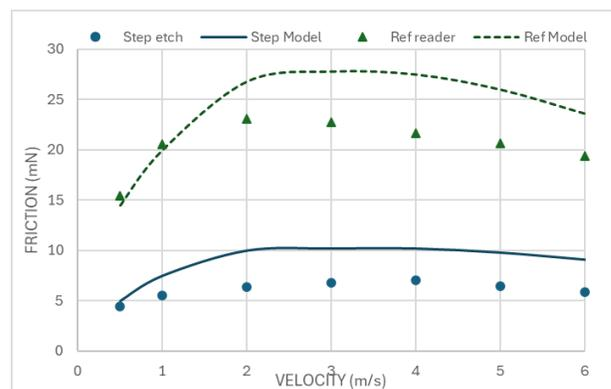
Fig. 3. Friction force as a function of tape velocity, at  $0.5^\circ$  wrap angle.
