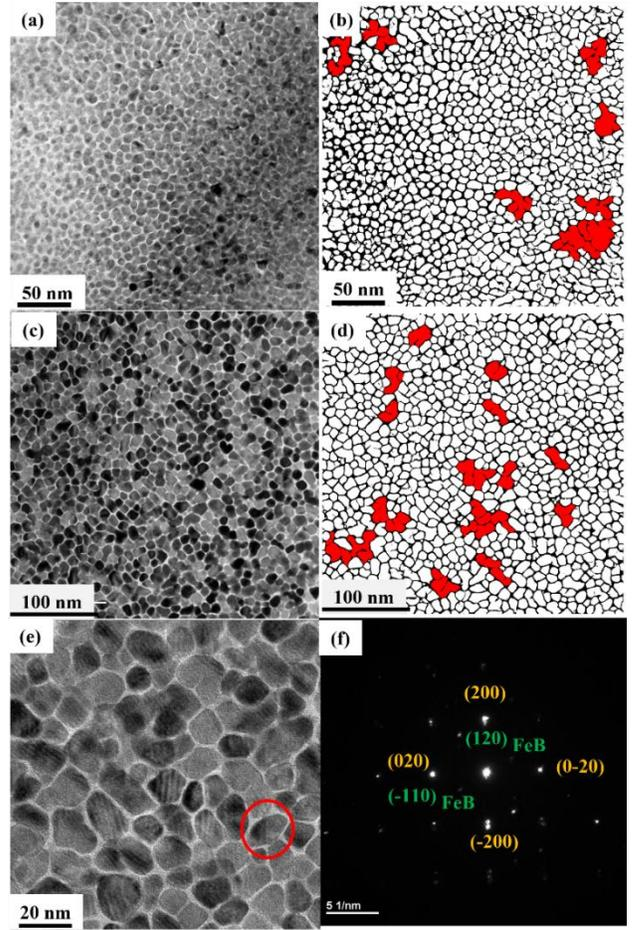
Fig. 4 The plane-view bright-field TEM images of (a) FePt(BN, Ag, C) film, (b) image segmentation of (a), (c) FePt(BN/AlN, Ag, C) film, (d) image segmentation of (c), (e) image with  $L1_0$ FePt-FeB grains (circle area), (f) nano-beam diffraction of circle area
