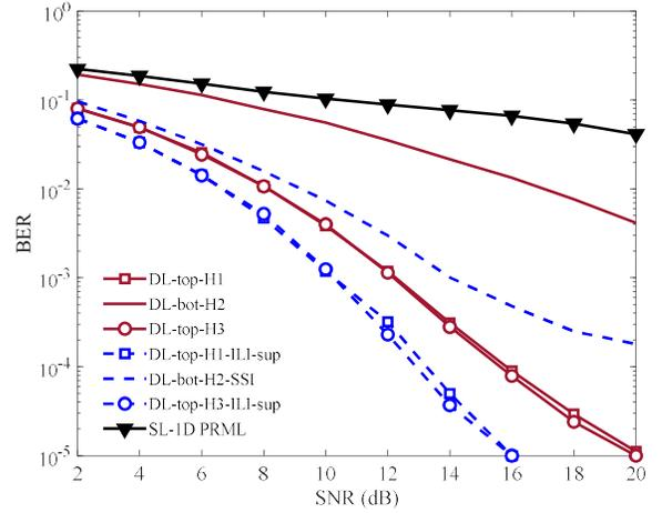
Fig. 3. Comparison of BER performance of SL- and DL-BPMPR systems.
