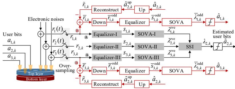
Fig. 2. The proposed dual-layer BPMPR channel model incorporates the SSI technique and the reproduced readback signal.
