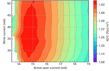
Fig. 3. A 2-D ADC map of head B. Compared with Fig.1 (b), it is less sensitive to write current.
