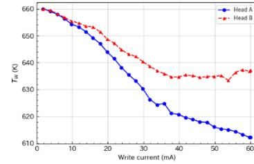
Fig. 4. Write current dependences of  $T_w$  calculated from THMap for two head designs. In  $T_w$  calculation, we assumed that  $T_c$  is 660 K.
