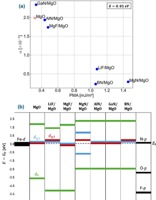
Fig. 1.(a). Relationship between PMA and  $\alpha$  for the pristine Fe/MgO and the interface modified model, Fe/MX/MgO. (b). Minority-spin  $d$ -orbital configuration by  $p$ - $d$  hybridization between the interfacial Fe and the adjacent anion (N, O, and F), for all models. Green, blue, and red represent  $d_0$  ( $d_{z^2}$ ),  $d_{\pm 1}$  ( $d_{xz, yz}$ ), and  $d_{\pm 2}$  ( $d_{xy, x^2-y^2}$ ), respectively.
