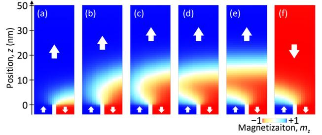
Fig. 3. Snapshots of the magnetic structure in the magnetization reversal process at time,  $t =$  (a) 0 ns, (b) 8 ns, (c) 16 ns, (d) 17 ns, (e) 18 ns, and (f) 24 ns. Each white arrow denotes the magnetization direction.
